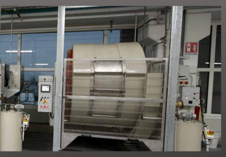
SOPRA E SOTTO ALCUNE VISTE DI BOTTALINI IN POLIPROPILENE COMPLETI DI BASAMENTO IN ACCIAIO, CANALA DI SCARICO, BIDI-NA PRODOTTI E IMPIANTO DI CONTROLLO TOUSCH SCREEN ABOVE AND BELOW SOME VIEWS OF POLYPROPYLENE DRUMS COMPLETE WITH STEEL BASE, OUTLET CHANNEL, PRODUCT TANK AND TOUSCH SCREEN CONTROL SYSTEM
