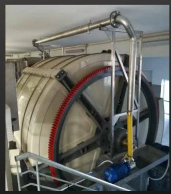
SISTEMA DI RISCALDAMENTO A RICICLO FORZATO CON POMPA FORCED RECYCLING HEATING SYSTEM WITH PUMP
