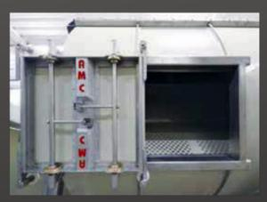
PARTICOLARE DELLA PORTA SCORREVOLE IN ACCIAIO INOX 316L RIVESTITA IN POLIPROPILENE DETAIL OF STAINLESS STEELE 316L SLIDING DOOR LINED IN POLYPROPYLENE
